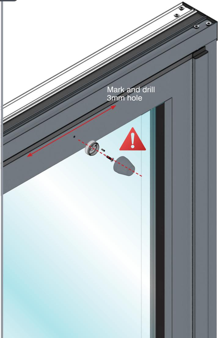
**Position grub screw opposite hinges and adjust angle to ensure magnets touching faces are parallel.**
